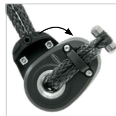
Cheek plates twist to open block
